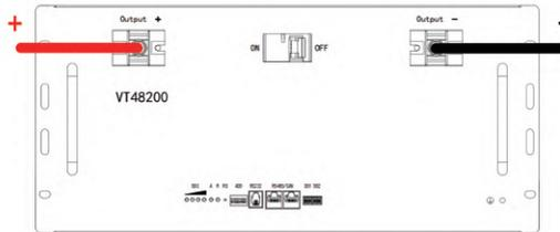
Figure 6-5 Connect the Battery Pack Power Cable
