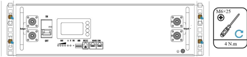
Figure 6-1 Install Battery Pack
