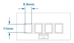
Figure 6 current cable terminal (Conductor Cross-sectional Area Range ≤16 mm<sup>2</sup>)
