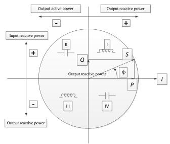
Figure 11 Measurement schematic diagram for energy four quadrants
