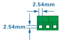
Figure 7 RS485 cable terminal (Conductor Cross-sectional Area Range 0.25-1mm2)
