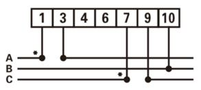
Figure 10 Three phase three wire: direct connect
