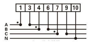
Figure 9 Three phase four wire: direct connect
