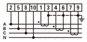
Figure 11 Three phase four wire: Connection throughcurrent transformers
