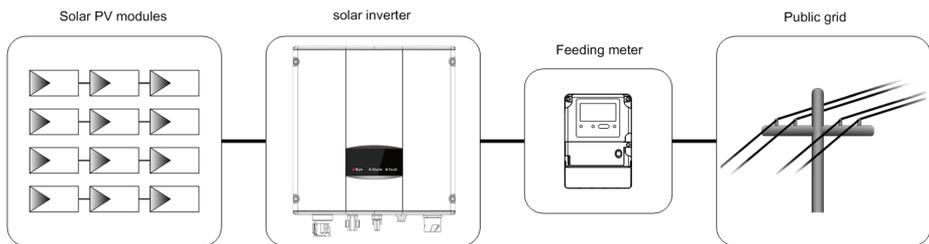
Figure 1 Application of the series grid-tied solar inverters
