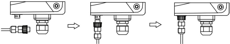
Figure 31 Detailed connectiona
