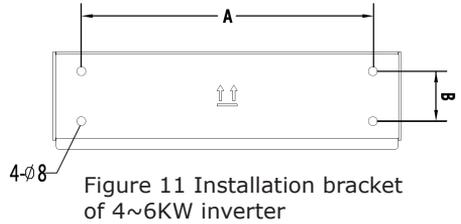
Figure 11 Installation bracket of 4~6KW inverter
