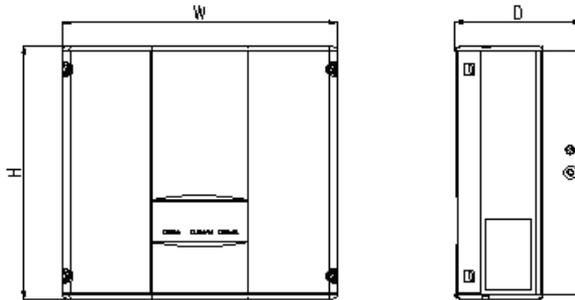
Figure 5 Inverter dimensions
