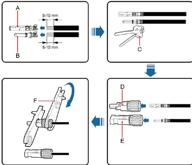
Figure 14 Connection between DC connector and solar modules
