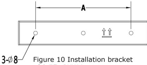
Figure 10 Installation bracket of 0.75~3KW inverter
