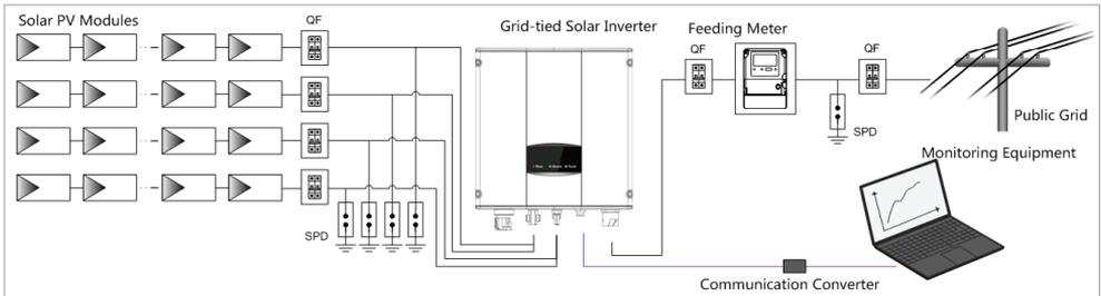
Figure 13 PV grid-connected system diagram
