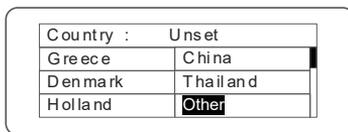
Press the "∧" or "∨" button to select the country (refer to the below table), press the ENT button to complete the setting.
