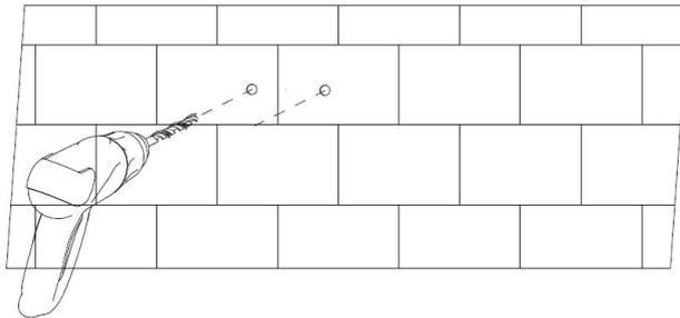
**Step 3:** Fix the hanging board. Clean the holes, use a rubber hammer to drive the expansion bolt into the hole, use a wrench to tighten the nut to fix the end of the bolt, then remove the nut, spring washer and flat washer, and then fix the wall mount plate to the wall and lock it with a tightening torque of 13N\*m. .
