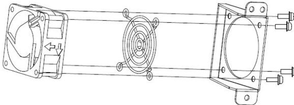
**Step 5:** Re-install the fan tray to the inverter in the reverse order and restart the inverter. .
