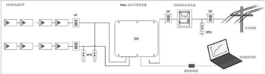
Fig 5.1 Schematic diagram of PV grid-connected system connection
