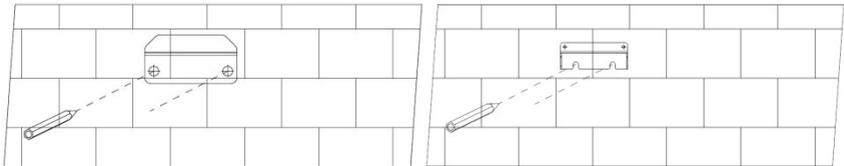
**Step 2:** Use a hammer drill to drill holes and install expansion bolts. Users need to prepare expansion bolts by themselves. It is recommended to use M8×60 stainless steel pressure explosion expansion bolts.
