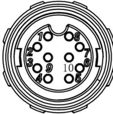
Fig 5.7 DRM & RS485 connector Front view
