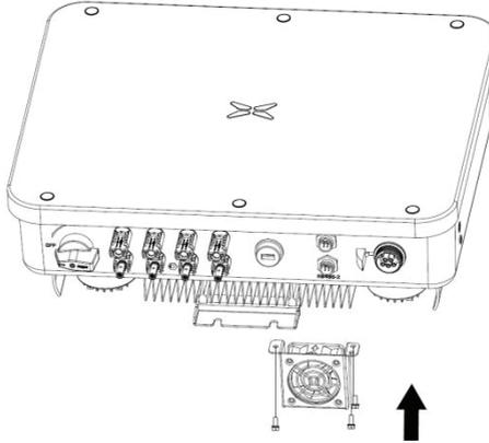
**Step 3:** Use a soft brush or vacuum cleaner to clean the fan. If the fan is damaged, follow step 4.
