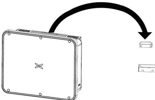
**Step 4:** Use an M4×12 screw to fix the inverter with the hole on the left side of the chassis and the wall mount, and the tightening torque is 2.5N\*m
