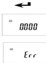
After entering the configuration data modification interface, short press the flip, can cycle query prompt of baud rate (bAU) , baud rate, prompt of address (Adr) , address, prompt of password (PSd) , password, clear energy prompt (CLr), clear energy command options.
